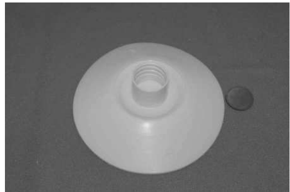
Base with gasket removed from center.
